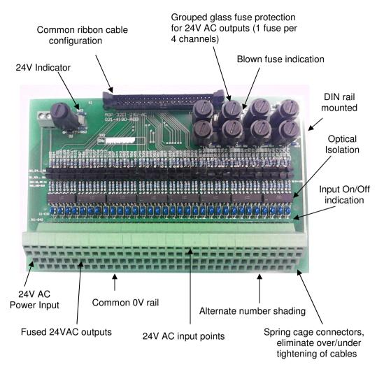
This product is designed to meet Council Directive 73/23/EEC low voltage, by applying the safety requirements EN 61131-2.
